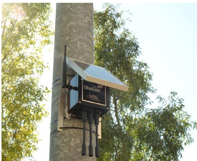
Figure 2.5 - Wasp mote Powered by Solar Panel
