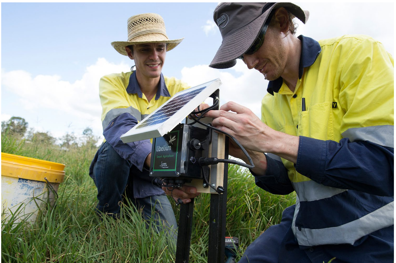
Figure 3.3 - Libelium sensors and EnviroSuite Agriculture Model being installed at AJ Bush
